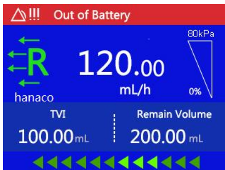
Figure 8-6 Out of battery alarm
