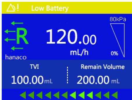
Figure 8-10 Low battery alarm
