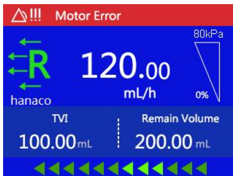
Figure 8-8 Motor error alarm
