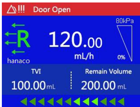
Figure 8-1 Door open alarm
