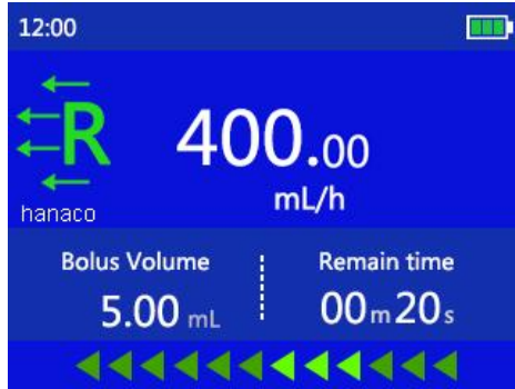
Figure 7-5-2 Bolus operation in progress
